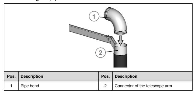
• Insert the elbow pipe (1) into the connector of the telescope arm (2).
