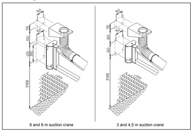
We recommend determining the assembly height of the suction crane as follows:
