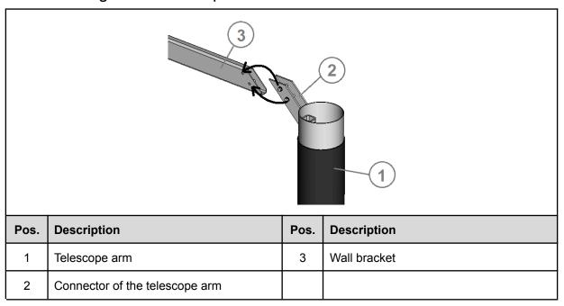
• Mount the connector of the telescope arm (2) at the outer end of the wall bracket (3). Use the supplied screws.
